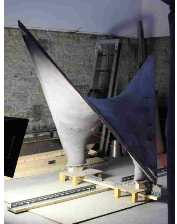
fig. 15 Prefabricated Hypar Component
