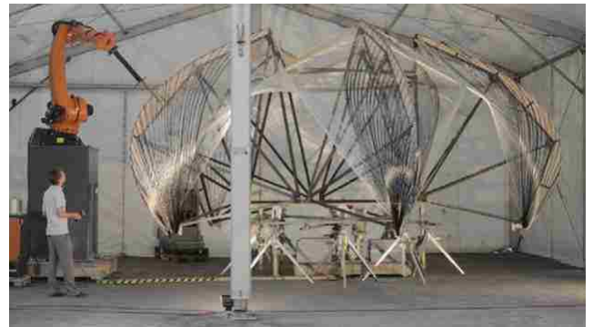
fig. 24 Continuous fabrication of fiber shell
