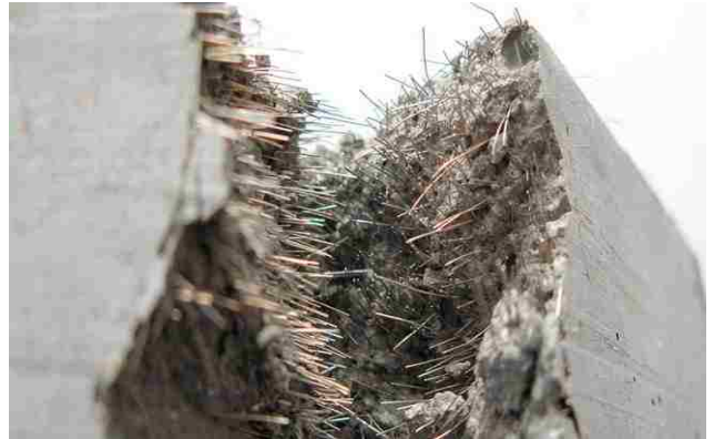
fig. 19 "Ultra-high performance", fiber-reinforced concrete
